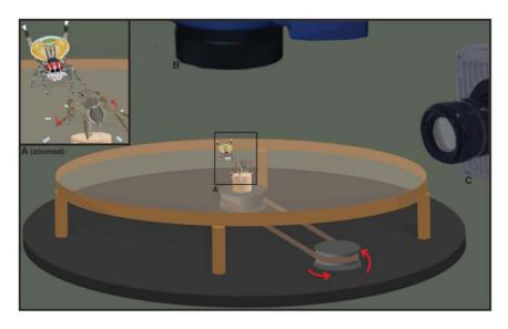
Figure 1. Courtship recording set-up. (A) Focal area for the regular speed camera (CV-S3200), (B) laser vibrometer (PSV-400) and (C) high-speed doi:10.1371/journal.pone.0025390.g001
